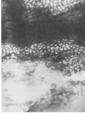
FIGURE 4. Transmission electron photomicrograph of a parallel section of an anodic oxide produced by 20 min CA/HF anodization at: 298 K, 20 A/m 2 , and 10 V (200,000 \times ).
